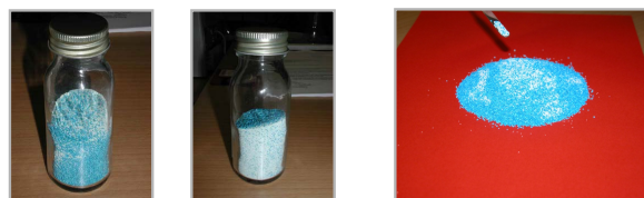
Figure 4. Illustration of the proverbial white powder with a normal grain-size distribution in which the larger-than-average particle sizes have been dyed blue, allowing detailed insight into grain-size differentiation and segregation behavior. The original powder visually makes a totally homogeneous impression. Shown here are two different DH_L manifestations (left, center). The powder state pictured center was produced by a single 90 degree rotation around the vertical axis of the container, attesting to significant DH_L handling sensitivity, illustrating that specific DH_L manifestations are always transient, a sensitive function of a number of factors (production, handling, transportation, manipulation while being sampled). This phenomenon applies to very many similar aggregate materials at all scales. The right hand illustration shows the effects of pouring segregation and the resulting problems acquiring a representative single-sample aliquot using a laboratory spatula. Discrete sampling (grab sampling) operations can never be representative. Illustrations courtesy of Peter Paasch-Mortensen (shown with permission).
