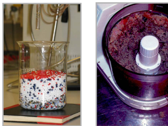
Figure 3. Left: Significant compositional and distributional heterogeneity of a composite material clearly related to its preceding laying-up (filling of the beaker). Sampling of this type of very irregular heterogeneity must cover all three sampling target dimensions, but may alternatively have taken place prior to, or simultaneously with an earlier transportation stage. Right: Significant compositional heterogeneity; here the end state resulting from thorough mixing of a batch of herring filets in a food processor. By using high-powered illumination and a camera UV-filter, hitherto invisible compositional differences among individual particles are emphasized, revealing an appreciable residual heterogeneity in what is normally called the homogenate.
