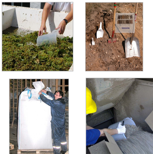
Figure 1. Primary manifestations of heterogeneous materials. Top left: Grab sampling (discrete sampling) of highly heterogeneous slurry (grapes/must) at a winery intake. Top right: Array of optional increment sizes for sampling of soil with intermediate heterogeneity. Lower left: Sampling targets as big bags offers the dubious complacency of not observing the material and its heterogeneity when sampling (but the heterogeneity very much exists nevertheless). Lower right: Manual process sampling (grab sampling) of apparently uniform material. The heterogeneity manifestations shown cover the range from high to low, from visible to hidden, from the considered to the neglected.
