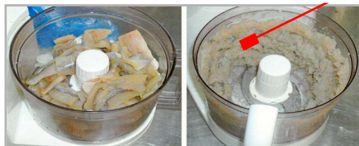
Figure 2. Primary manifestations of heterogeneous material in the laboratory. Here herring filets are subjected to sample processing and preparation before aliquoting. The food control laboratory in question believes that the resulting homogenate (right) is sufficiently well comminuted and mixed to allow direct aliquoting with a spatula (grab sampling), extracting only the precise, very small amount needed for analysis. The homogeneity is routinely assessed by visual inspection only; however, a Relative Sampling Variability characterization allows a fully quantitative heterogeneity characterization.
