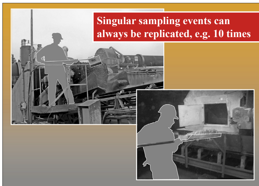
Figure 4. Examples of replication experiments (RE) that are easily set up. On the left is a dynamic process sampling situation, at the right sampling from a stationary lot. Both sampling scenarios can be assigned an objective RSV quality index. In order that no misunderstanding may occur, it is only necessary to perform a proper, calibrating RE once , as part of surveying and characterising the intrinsic heterogeneity of a specific lot material.
