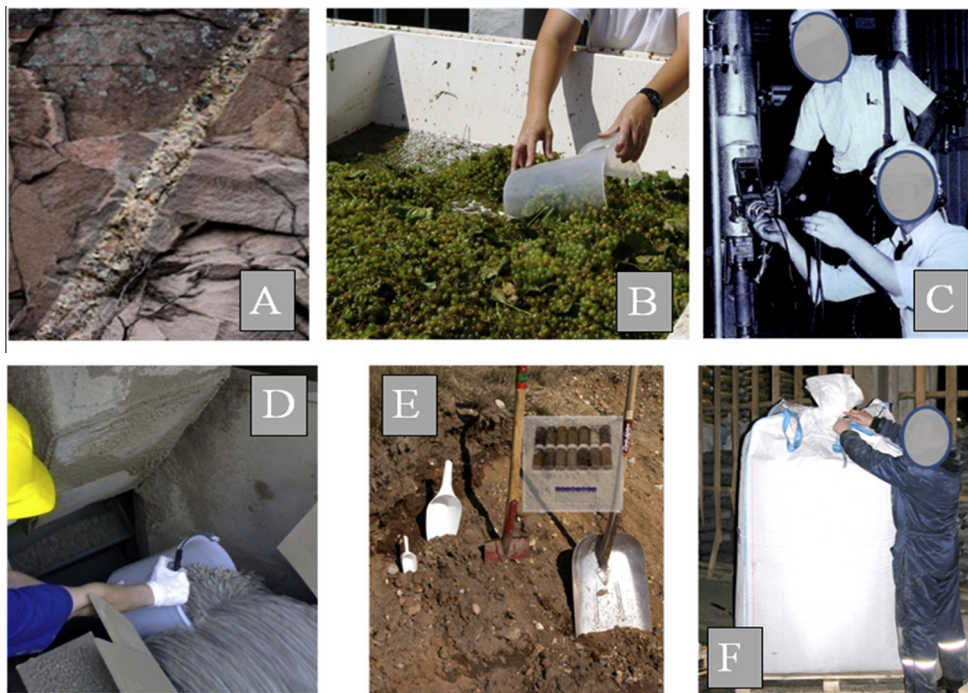
Fig. 3. Heterogeneity has infinitely many manifestations (selected examples shown here only). Material/lot heterogeneity can be structured (e.g., as in a pegmatite intrusion (dike) [A] or in glacial till (soil) [E]), invisible to the naked eye (i.e. 'uniform materials') at many scales (e.g., wine grapes [B] or lightweight expanded clay pellets ('LECA') [D]), or the state of heterogeneity can be hidden from observation (see also Fig. 4), as in the proverbial 'big bag' case [F] and [C], which shows a process analytical technology (PAT) probe insertion in a pipeline (process sampling).
